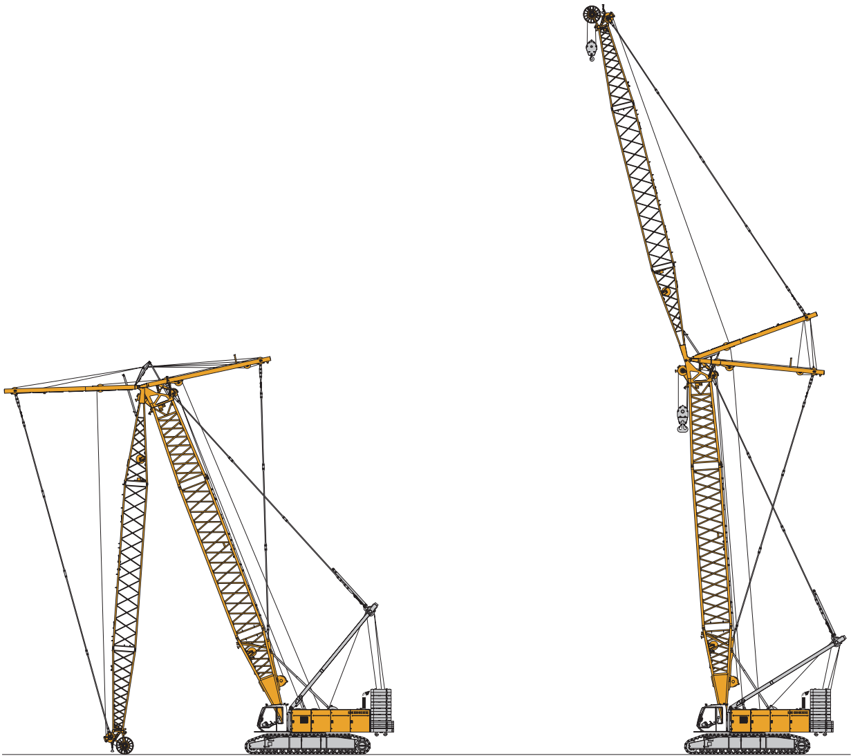
Erecting of main boom and luffing jib
